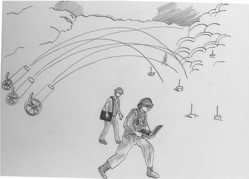
Figure 4. Hacker attack. Artillery shoots an infrastructure ad hoc network to the terrain enabling the mobile COTS nodes with omnidirectional antennas to join the network.
